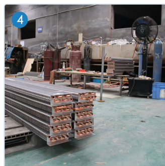
多回路盘管组装区 Multi-circuit Coil Assembly
