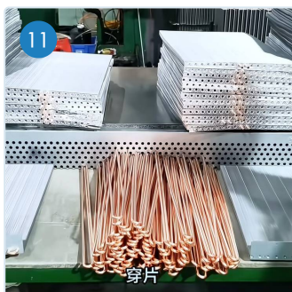
穿管半成品 Semi-finished Evaporator (Tube Inserted)
